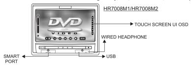
9) Pivot the screen until a comfortable viewing angle reached. The internal lock limits the screen to a maximum adjustment of 19 degrees from closed position, the headrest itself can be tilted forward to help achieve a comfortable viewing position.
